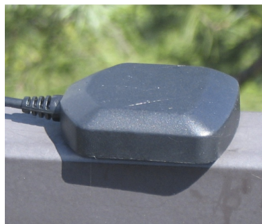
Figure 9.18 Active GPS antenna with housing. Dimensions: 46 x 39 x 12,5 mm. Usually a strong magnet at the bottom helps to attach such an antenna to a car-roof top or a similar metall surface.
