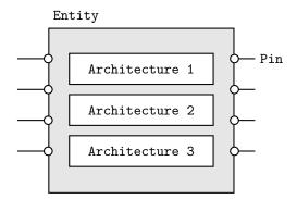
Entities are declared with port() that may contain a list of pins. Pins have a mode that can be in input (only LHS<sup>1</sup>), out output (only RHS<sup>2</sup>), inout bidirectional or buffer that can stay both on LHS and RHS. The usage of the latter is discourareged in favour of an internal signal.
