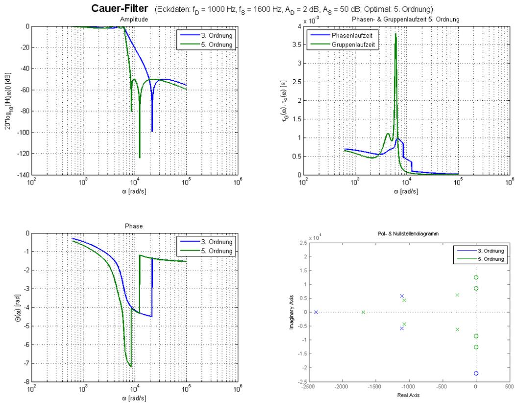
Cauer-Filter mit UTF  $H(s) = \frac{108.8s^4 - 6.596e-010s^3 + 2.538e010s^2 - 0.08009s + 1.29e018}{s^5 + 4398s^4 + 6.408e007s^3 + 1.939e011s^2 + 9.227e014s + 1.29e018}$
