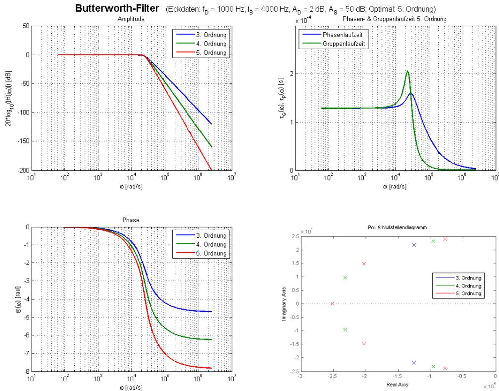
Butterworth-Filter mit UTF  $H(s) = \frac{1.003e022}{s^5 + 8.133e004s^4 + 3.307e009s^3 + 8.312e013s^2 + 1.291e018s + 1.003e022}$
