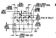
**RECOMMENDED PC** BOARD LAYOUT (Component Side)
